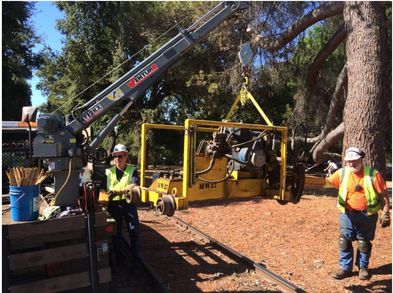
Ed and Frank use the truck's crane to get the section-gang machine off the track.
